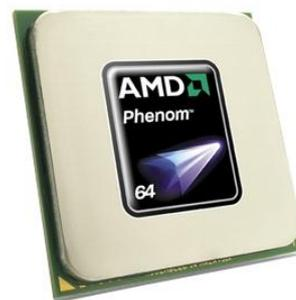
**Dual-core** processor has **two** cores (e.g. AMD Phenom II X2, Intel Core Duo)
